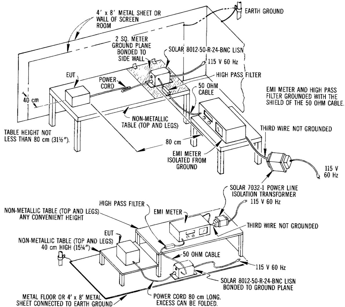
TYPICAL TEST SETUPS FOR CONDUCTED EMISSIONS
