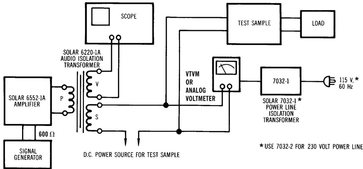
**AUDIO SUSCEPTIBILITY TEST SETUP FOR D.C. LINES**
