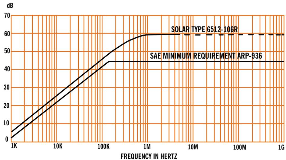
INSERTION LOSS MEASURED IN 50 OHM CIRCUIT PER MIL-STD-220A
