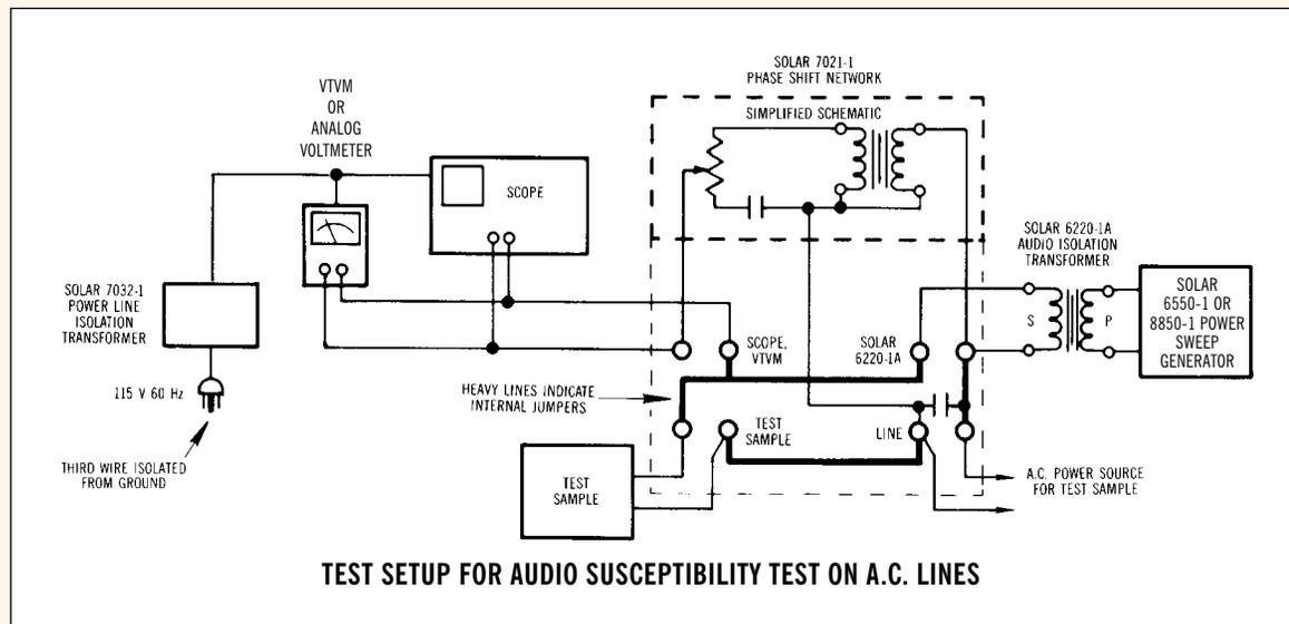
There is some interaction of these controls and when one is adjusted, the other should be readjusted and this action repeated several times. With careful attention to this, it should be possible to reduce the levels to below 300 millivolts on the voltmeter. Then, the audio source can be increased until the voltmeter indicates the voltage required by the susceptibility specification.
