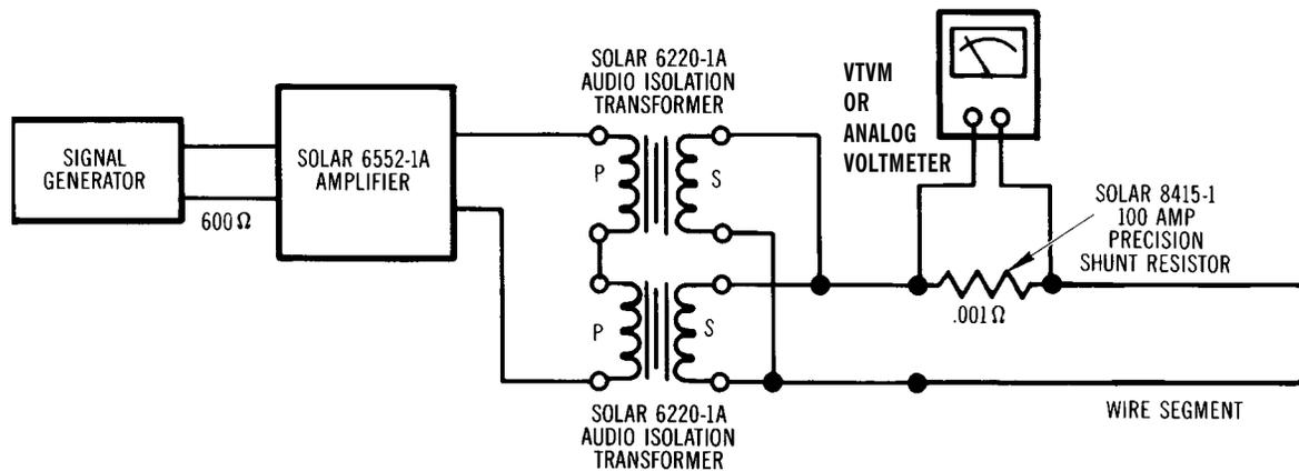
**SUGGESTED METHOD OF GENERATING UP TO 30 AMPERES IN WIRE SEGMENT FOR SHORT PERIODS, 20 Hz to 5 KHz**
