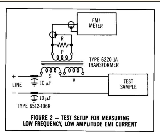
injection tests to prevent the transient from being short-circuited by the impedance of the power line. In this application all other windings are left open. See Figure 1. Secondly, the transformer can be used for measuring EMI current as described herein. See Figure 2. At other times, if it is not needed in the circuit, short circuiting the primary winding will effectively reduce the secondary inductance to a value so low that the transformer acts as if it isn't there.
